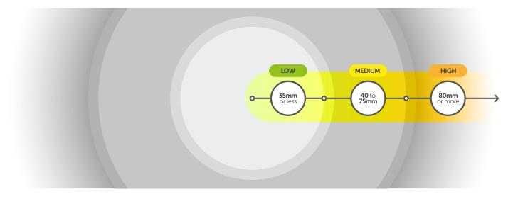
LOW radius of effects of ignition (up to 35mm) / MEDIUM radius of effects of ignition (40 to 75mm) / HIGH radius of effects of ignition (80mm or over)
