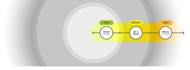
LOW radius of effects of ignition (up to 35mm) / MEDIUM radius of effects of ignition (40 to 75mm) / HIGH radius of effects of ignition (80mm or over)
